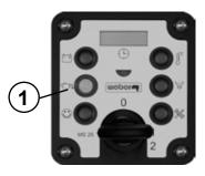
Charge level LED (1) is illuminated. Charging voltage too low or not available. Battery is not being charged.
